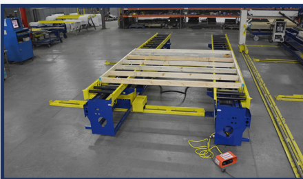
Wood Wall Squaring Station With Wall Panel
