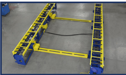
Wood Wall Squaring Station Without Wall Panel
