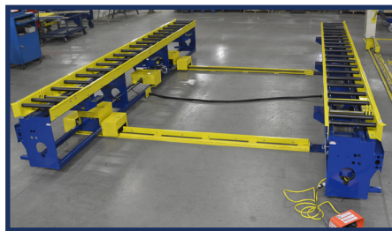
Wood Wall Squaring Station Without Wall Panel
