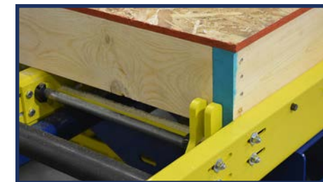
Wood Wall Panel Against Squaring Stops
