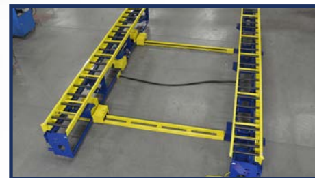
Wood Wall Squaring Station Without Wall Panel
