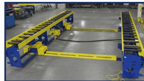
Wood Wall Squaring Station Without Wall Panel
