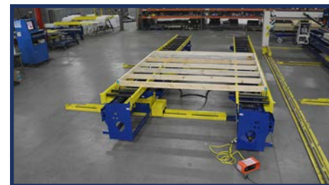
Wood Wall Squaring Station With Wall Panel
