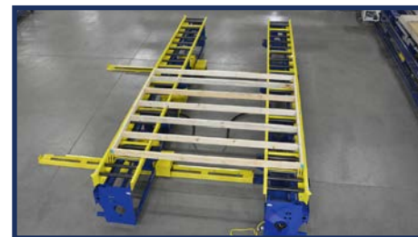
Wood Wall Squaring Station With Wall Panel
