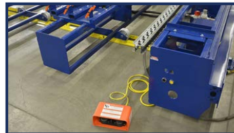
Footswitch & Push-Button Controls
