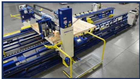
Single Tool Sheathing Bridge & Operator Platform
