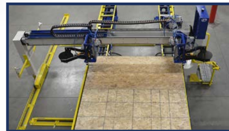
Single Beam Sheathing Station
