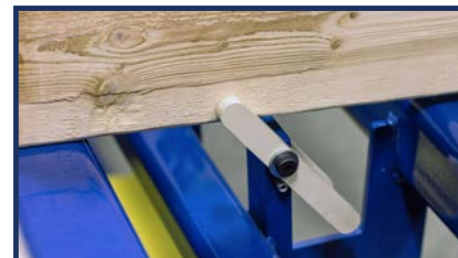
Color-Coded Stud Locators
