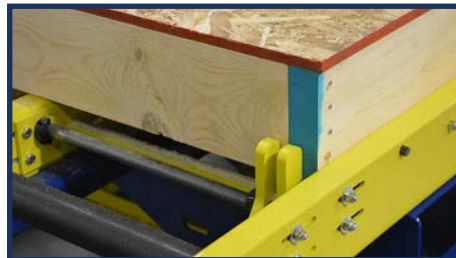
Wood Wall Panel Against Squaring Stops
