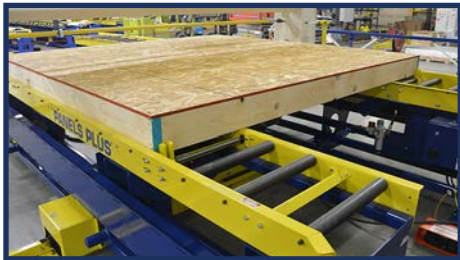
Squaring Table with Stationary & Telescoping Sides
