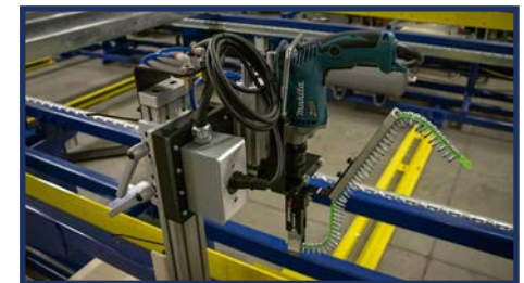
Screw Tool Carriage
