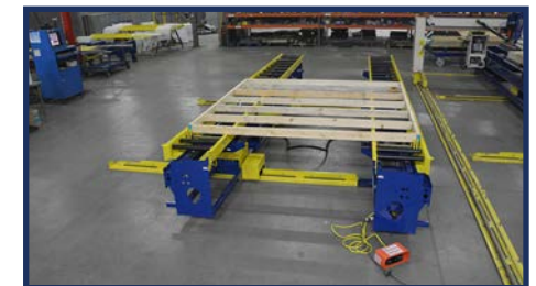
Wood Wall Squaring Station With Wall Panel
