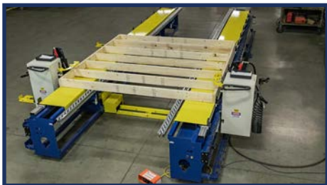
Wide Plate Framing Station With Indexing Tool Carriages
