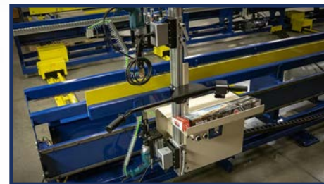
Framing Table with Screw Tool Carriage
