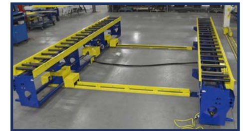
Wood Wall Squaring Station Without Wall Panel
