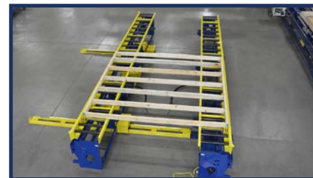
Wood Wall Squaring Station With Wall Panel
