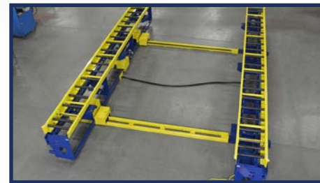
Wood Wall Squaring Station Without Wall Panel
