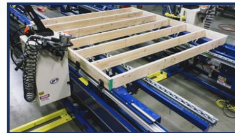
Framing Table with Indexing Tool Carriages
