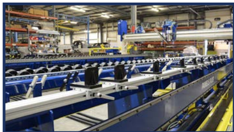
Color-Coded Stud Locators & Pop-Up Roller Conveyors
